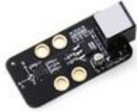
11012 Me 3-Axis Accelerometer and Gyro Sensor
