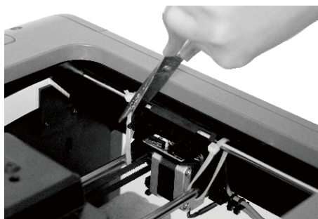
6. Use scissors to cut the four buckles that hold the rods in place.
