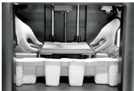
8. Hold on the platform, lift the build plate up with care.
