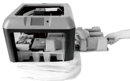
7. Remove the middle insert. A spool of filament is packed inside.
